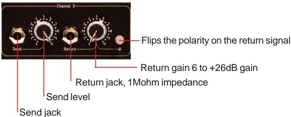
0dB balanced to +6dB unbalanced
