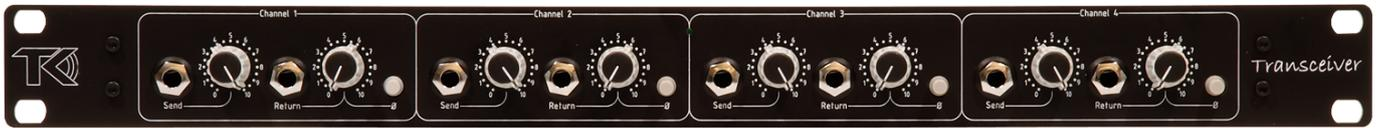
The Transceiver is a four channel universal interface between balanced and unbalanced gear. Each channel has a send level and a 0-20dB gain for the returns. A polarity switch is also provided on the return channels.
