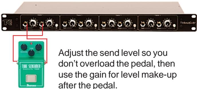
Adjust the send level so you don't overload the pedal, then use the gain for level make-up after the pedal.
