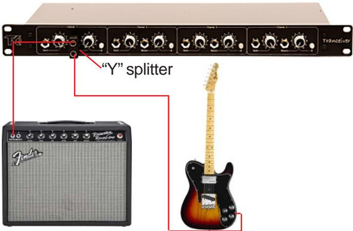
2. Lower the send level control and move the cable that feeds the amp to the send output instead. Now adjust the send control so you get the same amp level as you got when the amp was connected to the "Y" splitter. See picture to the right.
