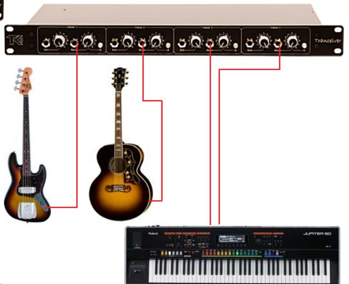
Because of its high input impedance it's a perfect DI-box for bass and passive instrument microphones.
