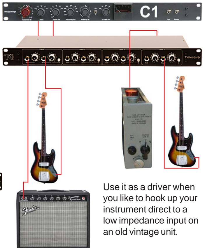
Use it as a driver when you like to hook up your instrument direct to a low impedance input on an old vintage unit.
